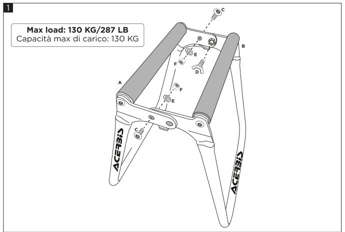
Position the (A) and (B) sides of the stand as indicated in the image. Insert the (D) wingnut and only tighten 3 turns leaving it loose. Insert the other 2 (C) bolts, the washers (E), and nuts (F) as indicated in the image and tighten them completely. Finish tightening the wingnut (D) until tight. To fold the up the stand, remove the wingnut (D).
